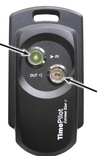
To clock out, gently tap the metal surface of your iButton to this probe. An orange light will flash inside the probe and the clock will beep to signal that you've been clocked out.
