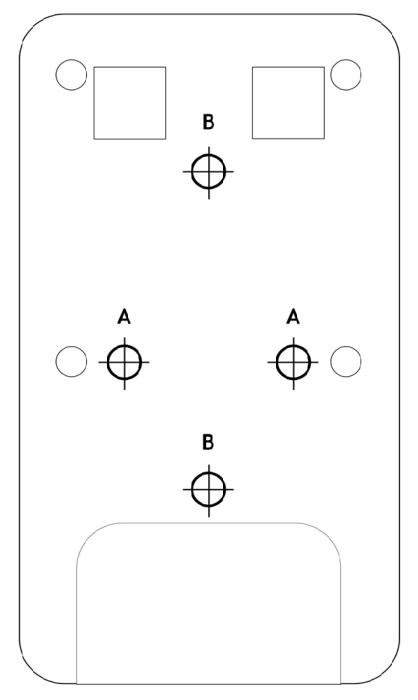
To easily mount the timeclock to a wall, attach this template to the wall and install the mounting screws where indicated by (Use the holes marked "A" if you're using the included wall anchors or mounting to an empty junction box; use the holes marked "B" if you're mounting to a stud.)
