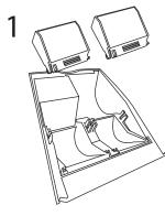
2 Put two rolls of thermal paper into each Both rolls must feed forward from underneath the roll.
